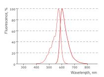
TurboFP602 normalized excitation (thin line) and emission (thick line) spectra.
